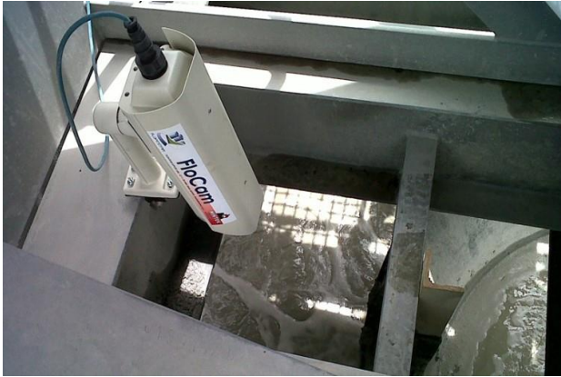
FloCam: A machine vision froth monitoring system
